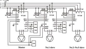
Control 5 auxiliaries at most, up to 6 pump linkage work
